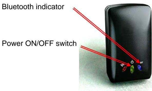
**Push the power switch 1~2 seconds to Power on**
